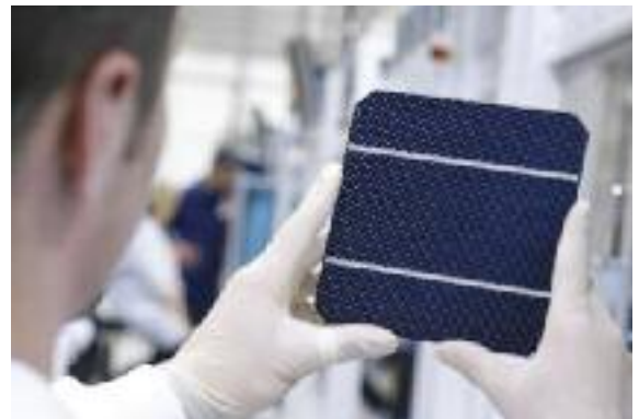
Monocrystalline solar cell.
