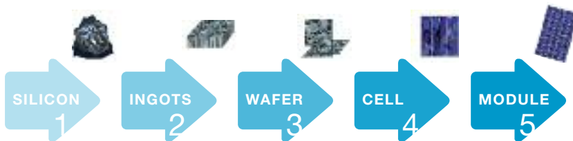
FIGURE 8 CRYSTALLINE SILICON MANUFACTURING PROCESS
